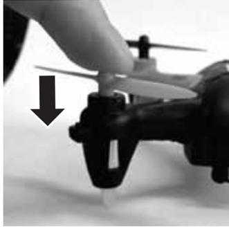
Blades must be installed as shown:
